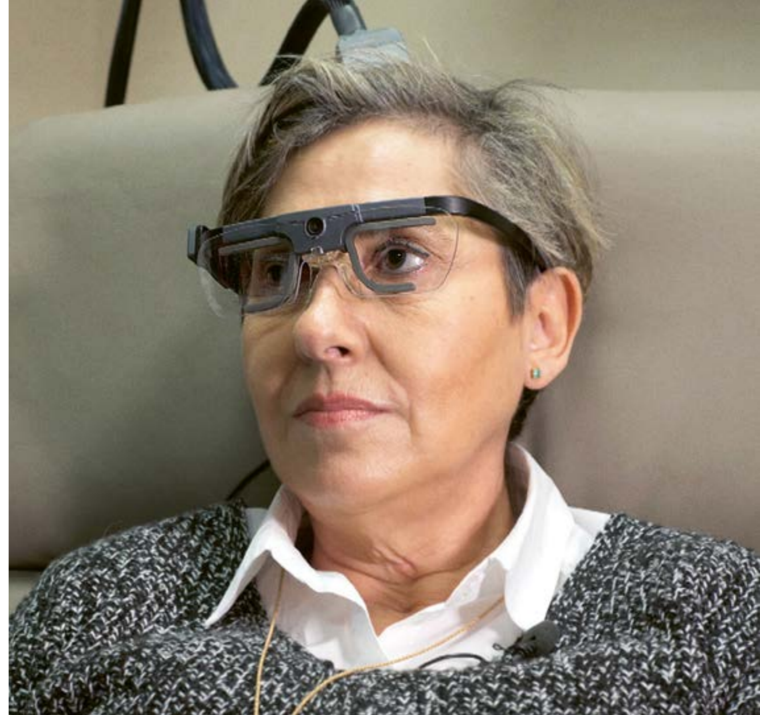
A miniature camera connected to an eye tracker built into the frame of glasses transmits visual information to the brain implant.
