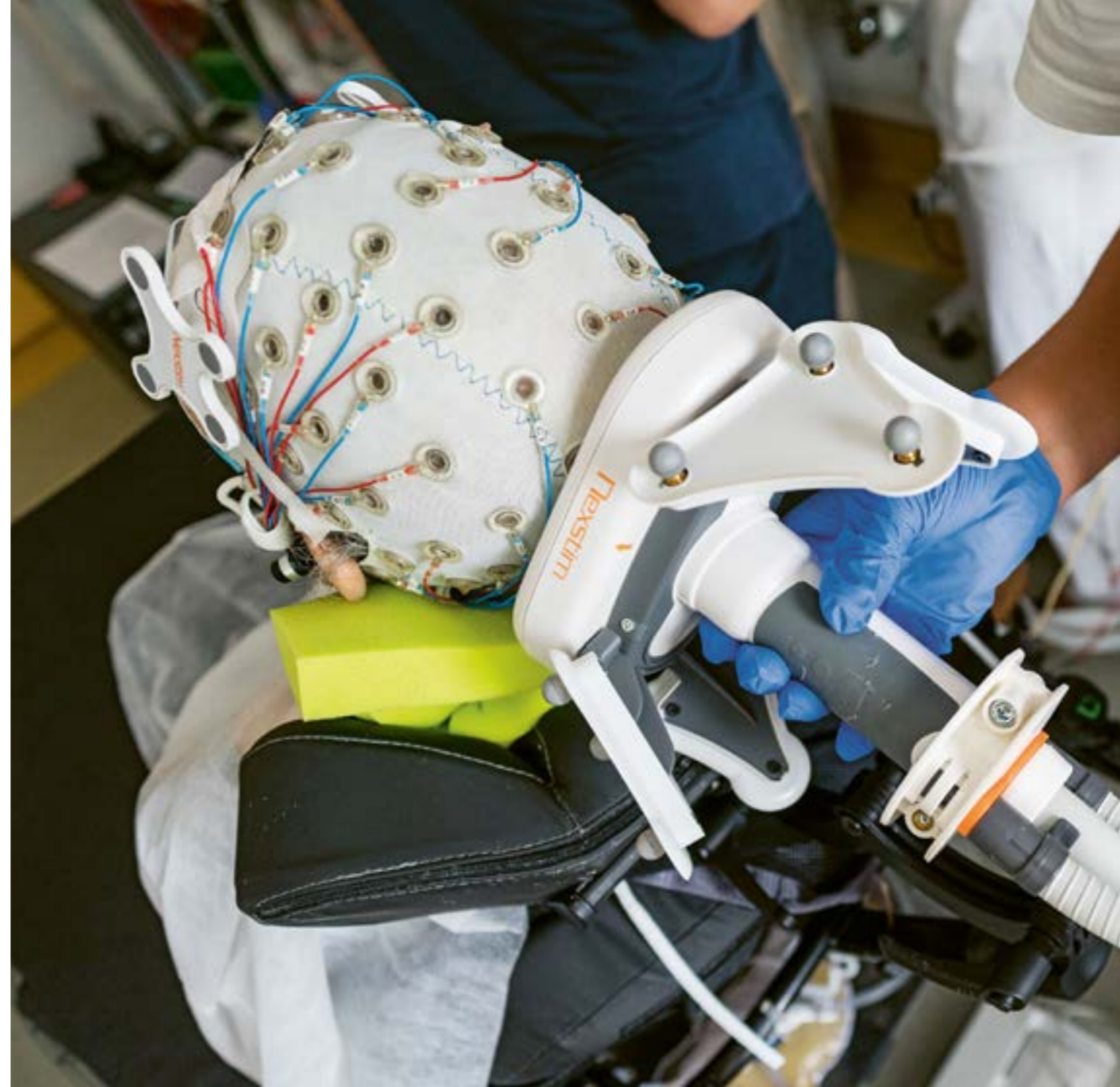
Magnetic stimulation and EEG readings are used to measure a patient's level of consciousness.
